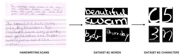
Figure 1: Raw handwriting data in the form of scanned pages are preprocessed and converted into two datasets: words and characters.
